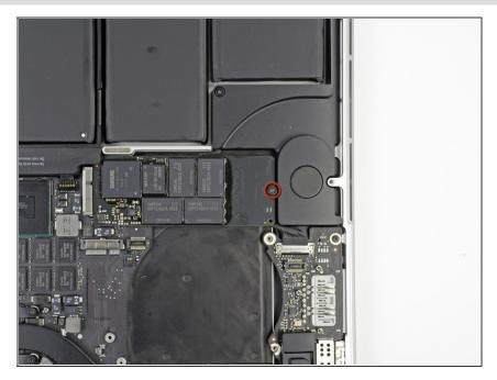
Remove the single 3.1 mm T5 Torx screw securing the SSD to the logic board.
